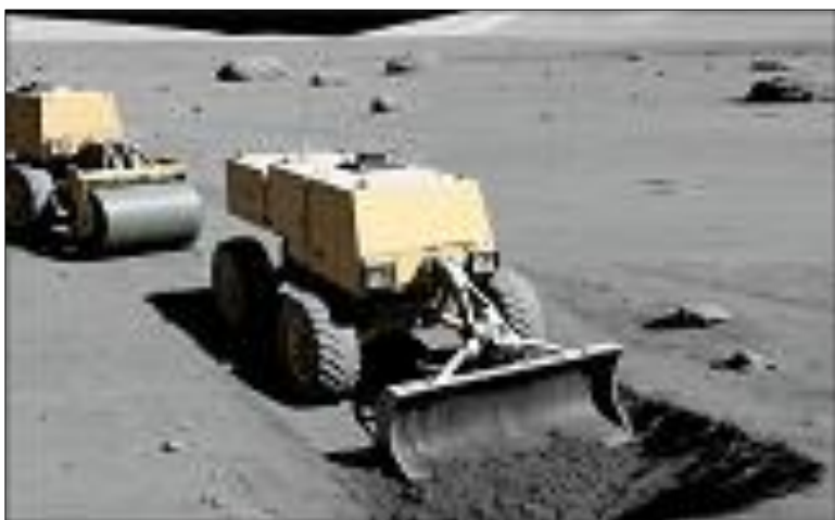
Teams of RoadBots autonomously constructing compacted dirt roads.
